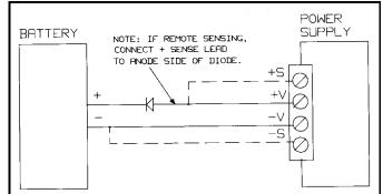
Figure 4-10. Recommended Protection Circuit for Battery Charging
